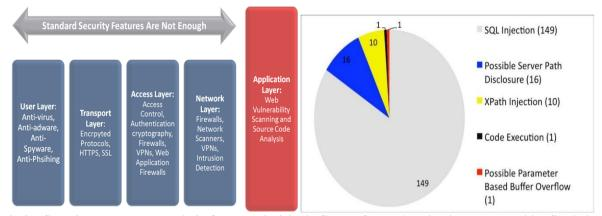
Fig 2.1 Security Layers as a Holistic OutlookFig 2.2 Pie Chart of Web Application Vulnerability Statistics 2010-2013
